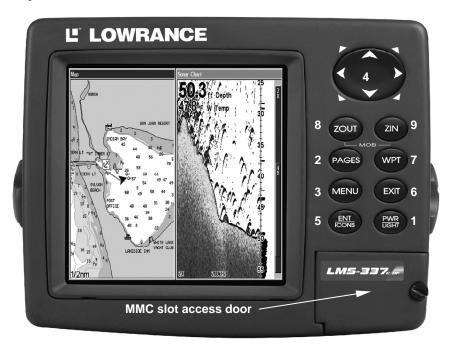
LMS-337CDF sonar/GPS unit, front view, showing map with sonar split screen, keyboard and access door for the MMC slot.
